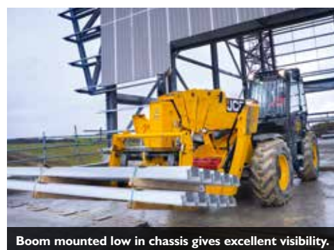
Formidable forward reach capability means the 540-200 can reach across typical building foundations with ease.
